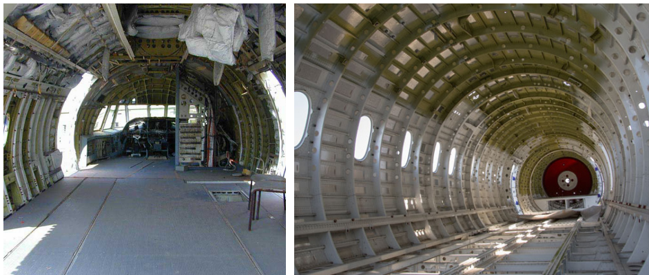
Left: cockpit emptied during the recycling process / Right: back 'semi-monocoque' fuselage of an Airbus A340 under construction
